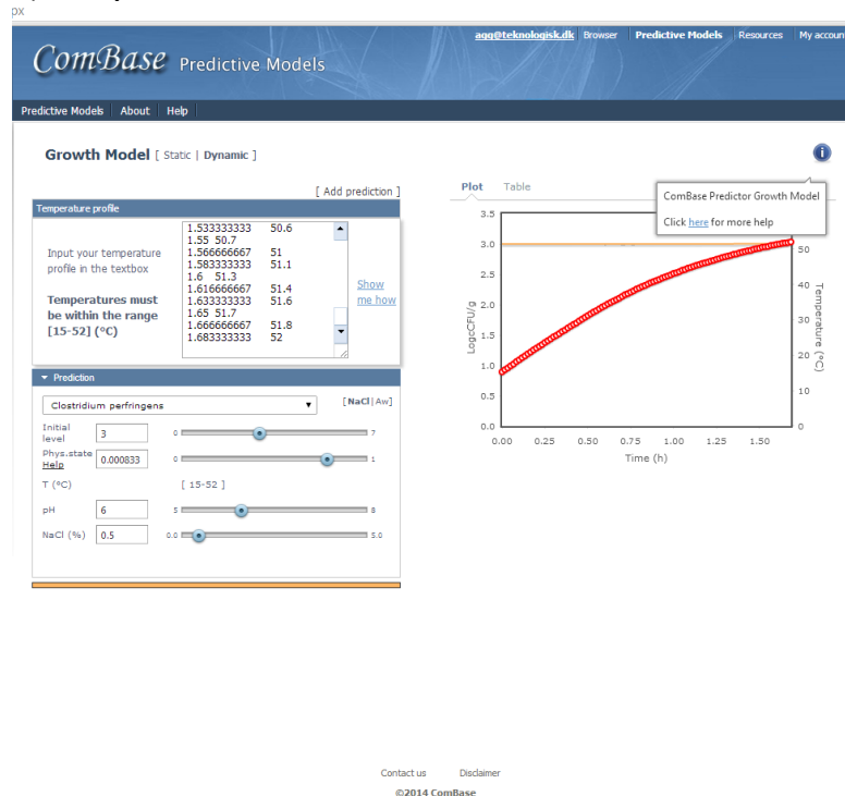
Figur 1. Output fra C. perfringens model i Combase Predictive models for temperaturprofil for opvarmning af skinke (d=6,0-6,5 cm)
